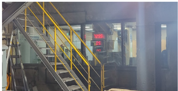
Installing triple soundproof glass to reduce noise from the electric furnace's operation room
